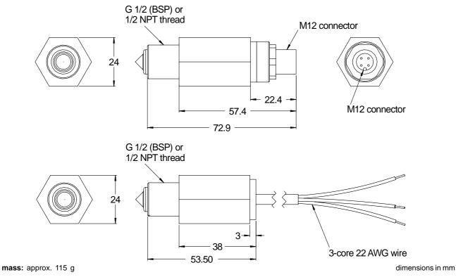
**Note:** Do not mount the sensor with prism pointing downwards.
